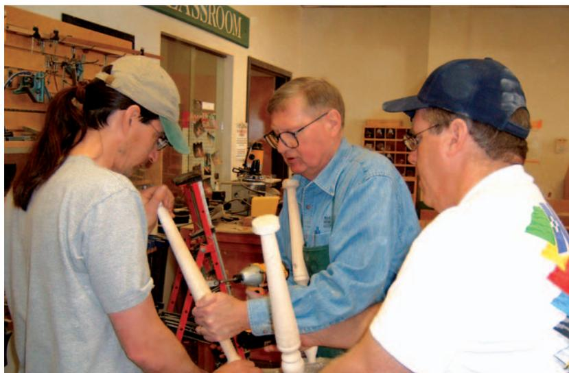
**DRILLING HOLES FOR THE LEGS** turned out to be a three-person job, one to drill and two to visually align the legs.
