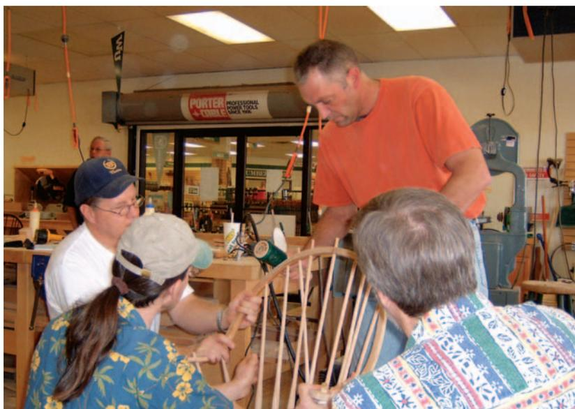
**GLUING UP THE BACK**, with its 16 components, was an eight-handed process. Students help each other make the perfectly spaced back to this continuous arm chair.
